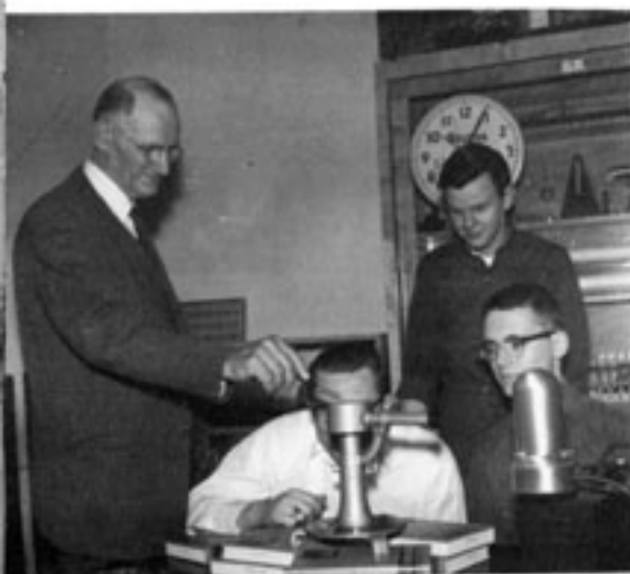
Physics students observe bright line spectrum with a sodium light by means of a spectroscope.
